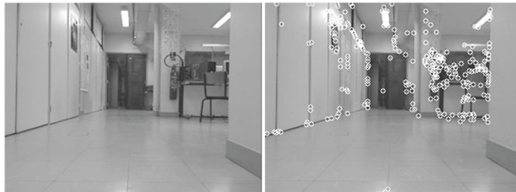
Figure 1 Image (320 × 240 Pixels) of the embedded camera and result of the FAST detector.
