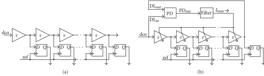
FIGURE 3: TDC based on (a) open-loop, and (b) closed-loop delay line.
