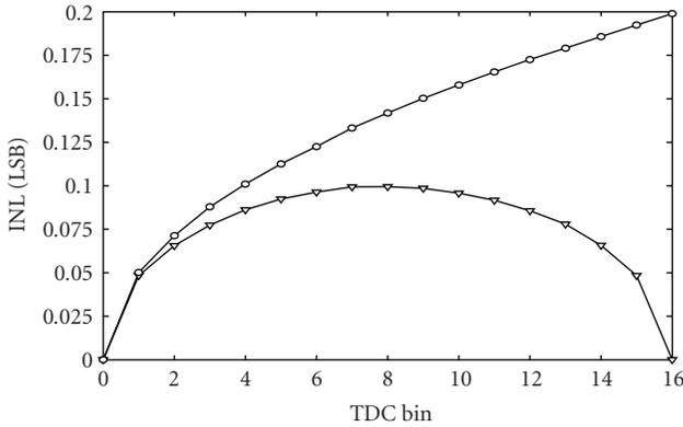
FIGURE 4: Simulated INL of a TDC based on an open-loop line (circles) and on a closed-loop line (triangles).
