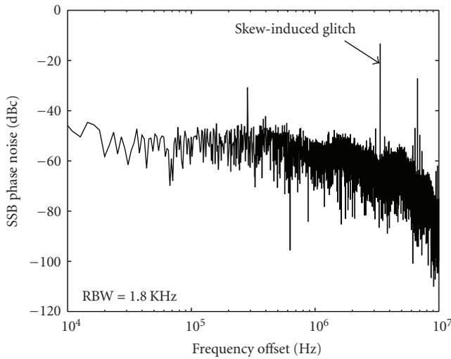
FIGURE 11: Output spectrum of the AD-PLL when the glitch corrector is disabled. The dominant spur is induced by the time skew between counter and TDC.
