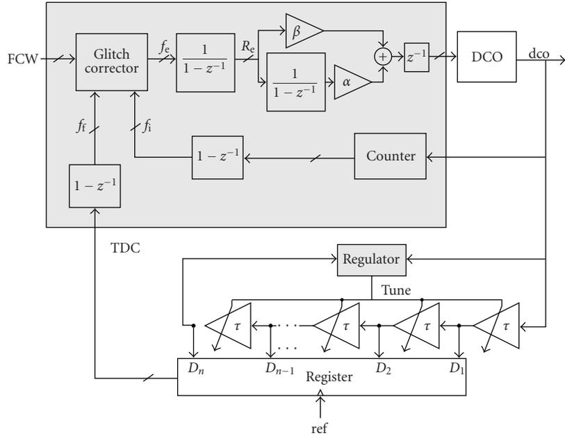
FIGURE 10: Full block schematic of the designed AD-PLL.
