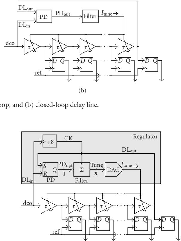
FIGURE 5: Schematic of the DLL-based TDC with bang-bang phase detector.
