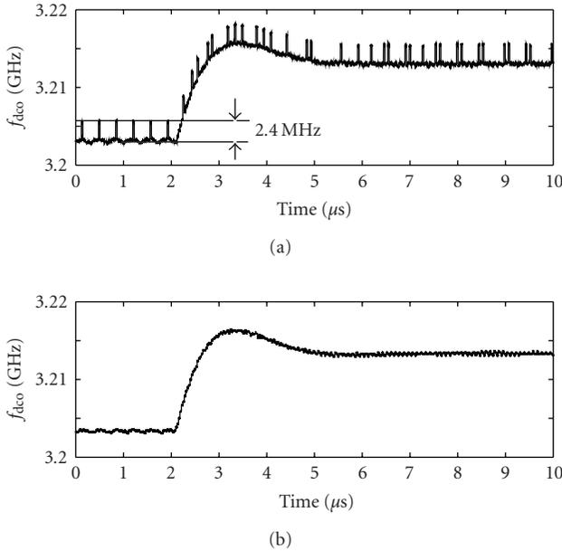
FIGURE 13: AD-PLL output frequency for a 10 MHz input step, when the glitch corrector is disabled (a) and enabled (b).
