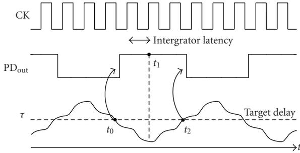
FIGURE 6: The limit cycle in the DLL.
