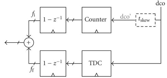
FIGURE 7: Time skew between the counter and TDC input signals.
