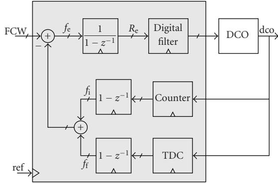
FIGURE 1: The AD-PLL block schematic.
