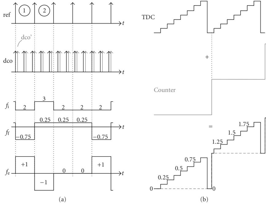
FIGURE 8: AD-PLL behavior for  $FCW = 2.25$  in the presence of a time skew between counter and TDC: (a) positive edges of  $ref$  and  $dco$ ,  $f_i$ , and  $f_e$ . (b) Counter/TDC conversion characteristic.
