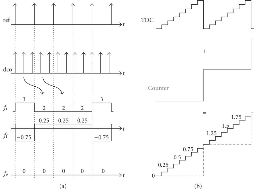
FIGURE 2: AD-PLL behavior for  $FCW = 2.25$ : (a) positive edges of  $ref$  and  $dco$ , feedback signals  $f_i$  and  $f_r$ , and error signal  $f_e = FCW - (f_i + f_r)$ ; (b) counter/TDC conversion characteristics.
