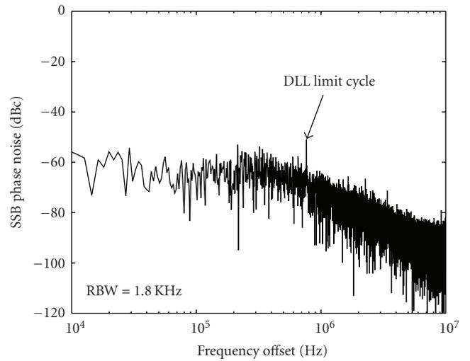
FIGURE 12: Output spectrum of the AD-PLL when the glitch corrector is enabled. The dominant spur is induced by the DLL limit cycle and it is below  $-50$  dBc.
