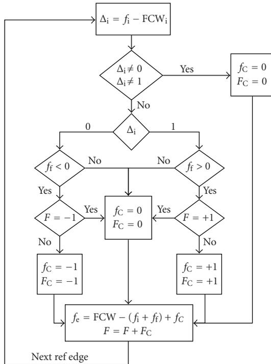
FIGURE 9: Flow chart describing the operating principle of the glitch corrector when  $0 \leq FCW_f \leq 0.5$ .
