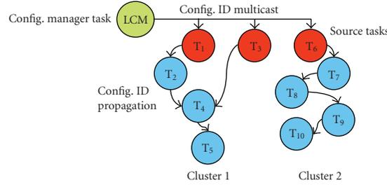
FIGURE 5: Synchronization with multicasting and propagation.
