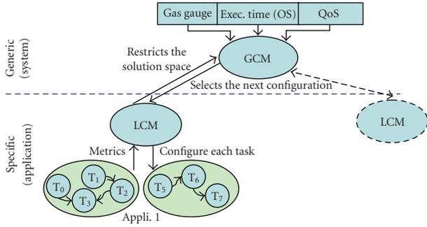
FIGURE 3: Application versus system configuration management.
