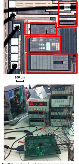
**Fig. 11** Picture of the die and of the measurement setup and evaluation board
