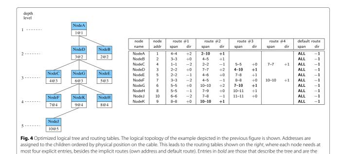
only ones considered to forward packets. The other entries were added to allow direct communication between nodes within direct visibility
