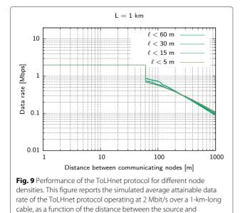
destination nodes. At this baud rate, direct communication is possible only up to about 60 m, then intermediate hops are needed, causing a
