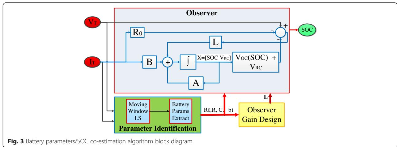
**Fig. 3** Battery parameters/SOC co-estimation algorithm block diagram
