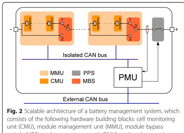
**Fig. 2** Scalable architecture of a battery management system, which consists of the following hardware building blocks: cell monitoring unit (CMU), module management unit (MMU), module bypass switch (MBS), pack management unit (PMU), and pack protection switch (PPS)
