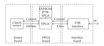
FIGURE 4: High-speed camera system principle.
