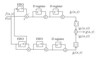
FIGURE 21: Optimized cascade Sobel filter implementation.
