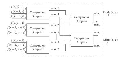
FIGURE 22: Schematics of erosion and dilation calculation.
