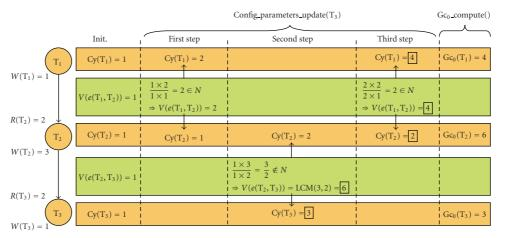
FIGURE 6: Gc<sub>0</sub> computation example.
