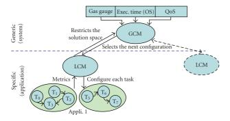
FIGURE 3: Application versus system configuration management.
