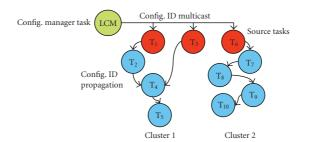
FIGURE 5: Synchronization with multicasting and propagation.
